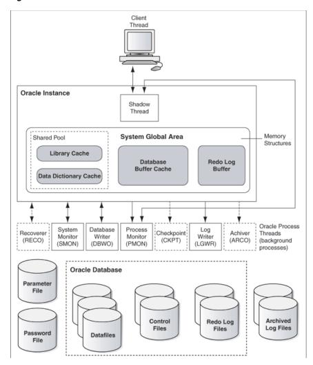
Figure 1–1 Oracle Database Architecture on Windows
