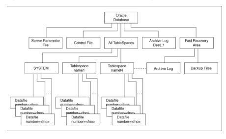
Figure 8–1 Oracle VSS Writer Component Hierarchy
