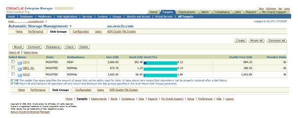
Figure 13–5 shows Enterprise Manager reporting a pending REBAL operation on the DATA disk group. The operation is almost done, as shown in % Complete, and the **Remaining Time** is estimated to be 0 minutes.
