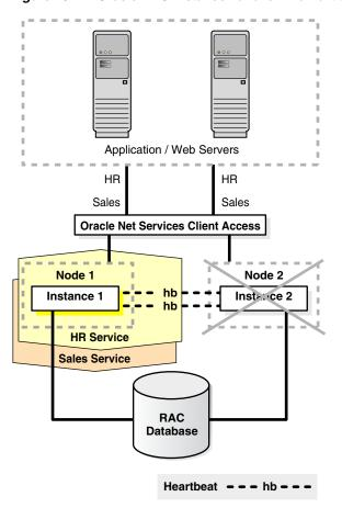
Figure 13-7 Oracle RAC Instance Failover in a Partitioned Database
