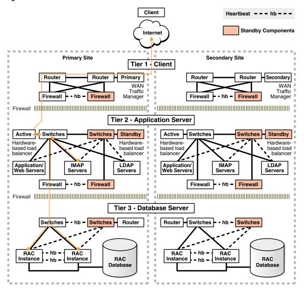
Figure 13–2 illustrates the network routes after site failover. Client or application requests enter the secondary site at the client tier and follow the same path on the secondary site that they followed on the primary site.
