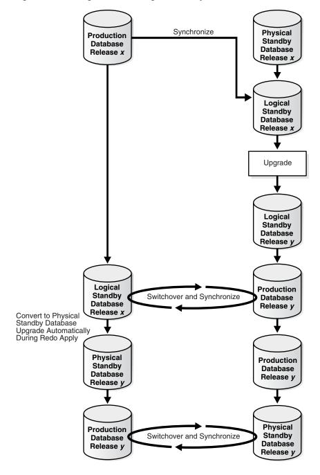
Figure 14–1 Using a Transient Logical Standby Database for Database Rolling Upgrade
